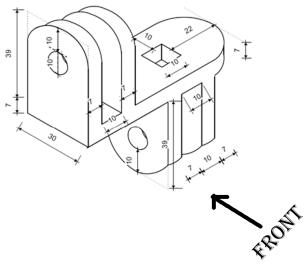
Draw the Plan, Front elevation, right and Left side elevations of the given object shown above, according to the measurement given (show hidden lines as dotted). All dimensions are in mm only.
